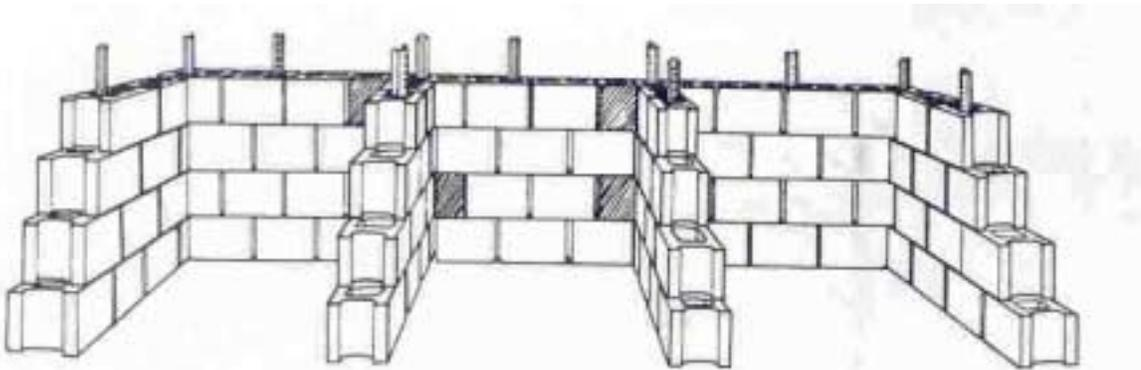
1. Place five concrete blocks in a row along the ground at the composting site, leaving about  $\frac{1}{2}$  " between each block to let in air.
