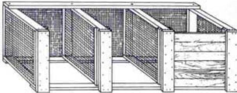
1. Cut two 31½-inch and two 36-inch pieces from a 12-foot length of pressure treated 2x4 lumber. Butt joint and nail the four pieces into a 35x36-inch square. Repeat, building three more frames with the remaining 12-foot length of 2x4 lumber.
