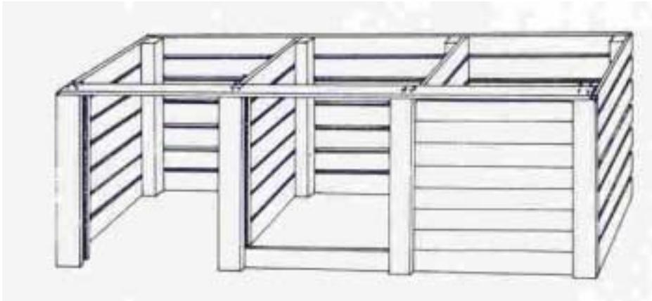
1. On level ground, set the posts using a posthole digger. Embed each post at least 2 feet into the ground. Be sure all posts are plumb (perpendicular to the ground). The top of each post should be at the same distance above the ground.
